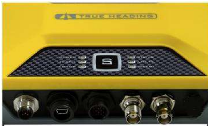
Figure 7. CTRX Graphene: From L to R: NMEA2000 connector, USB-mini connector, Data/DC circular connector, GPS antenna (TNC), VHF antenna (BNC).
