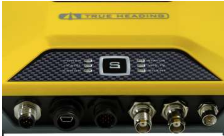
Figure 7. CTRX Graphene+: From L to R: NMEA2000 connector, USB-mini connector, Data/DC circular connector, GPS antenna (TNC), VHF antenna (BNC) and VHF radio (FME).
