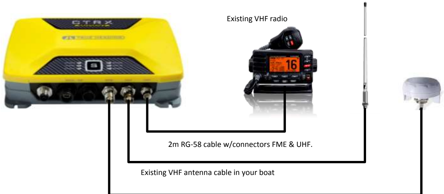
Cable, 5m, RG-58, attached to the GPS antenna
